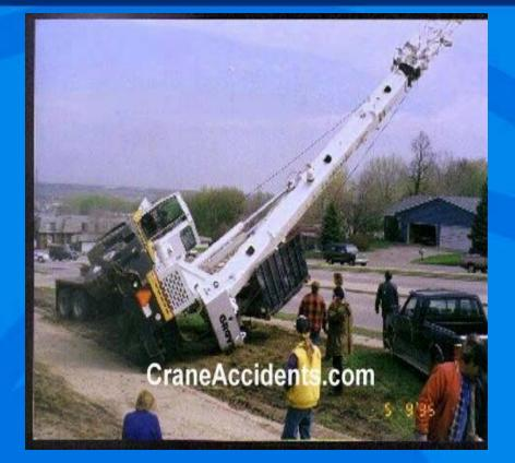
Two Leading Causes: Stability – tip & Structural – bends / breaks
